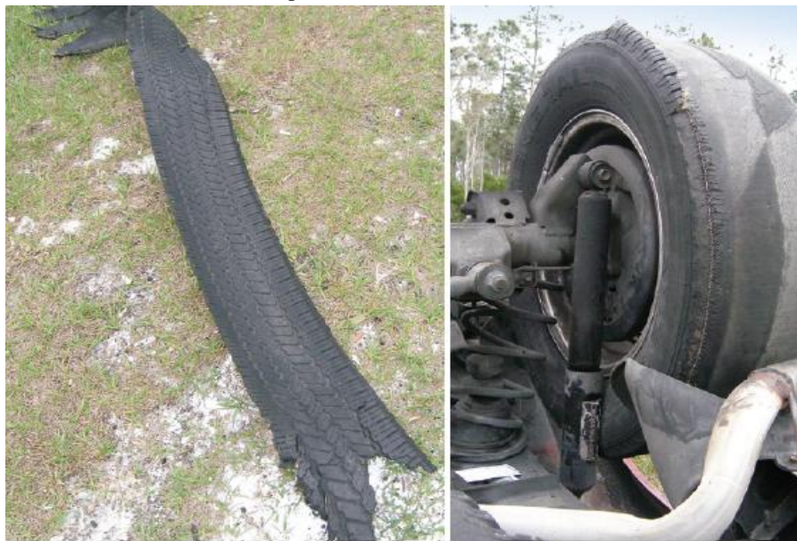
Figure 2. Tire treads Separation.
