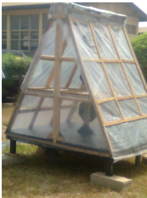
Figure 5 Pictorial view of a solar tent dryer equipped with a solar chimney
