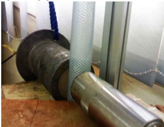
Figure 3: Gamma source and NaI(Tl) detector mounted on the test section
