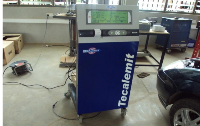
Figure 13 The Four-gas exhaust analyser used for the one-speed emissions test
