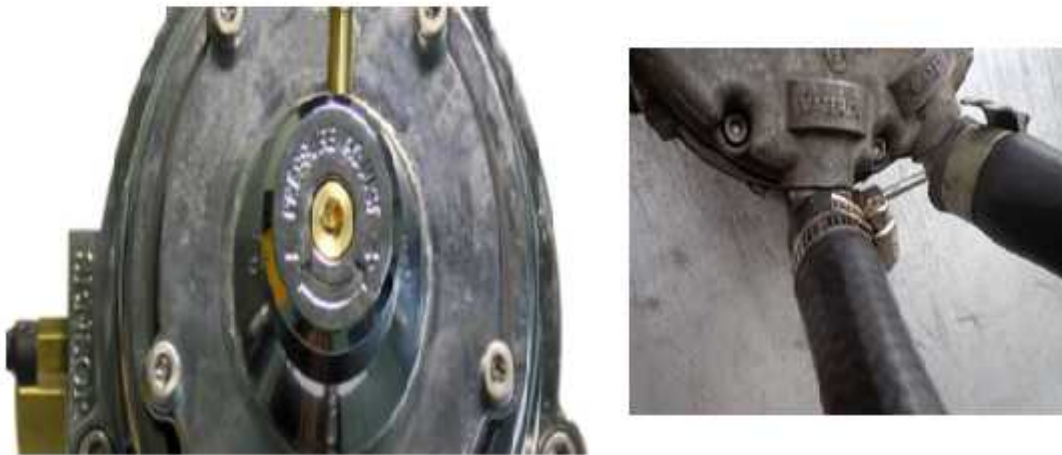
Figure 4: Vaporizers (left-with a temperature sensor and right-without a sensor)
